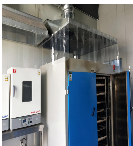
实验室硫化机集气罩
